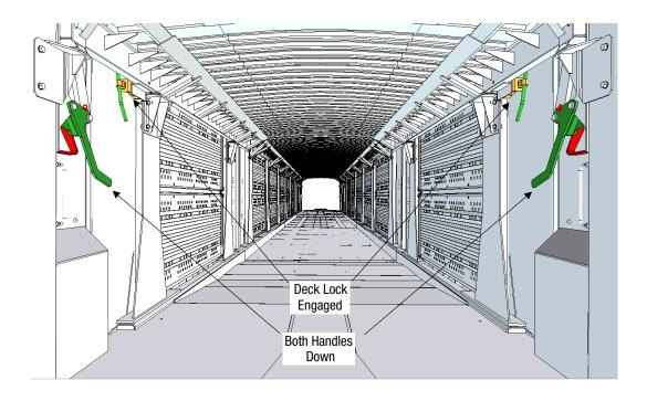
Pull the Deck Lock Lever to unlock the Deck Lift Handle.
