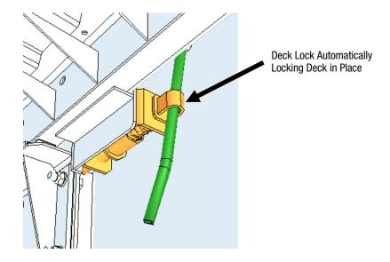
Inspect the deck to ensure it is completely resting on the Deck Supports. If it is not, make sure the Deck Lift Handle is pulled all the way down.
