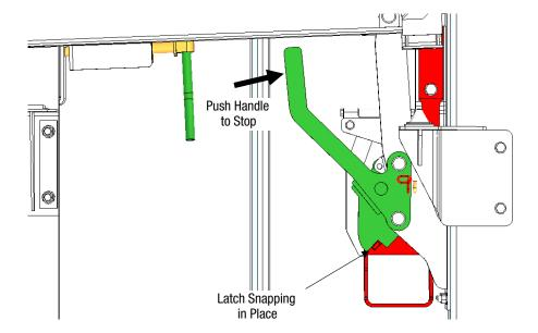
Inspect the Latch to insure it is fully engaged. The Latch should be pressed tight against the back of the Deck Lift Handle with very little clearance. If it is not, make sure the Deck Lift Handle is pushed all the way up and pull Latch Handle until it is tight against the Deck Lift Handle.
