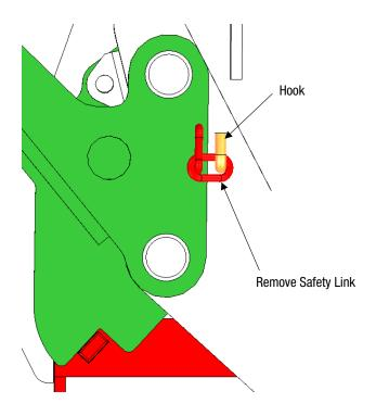
Push the Latch outward to unlatch the Deck Lift Handle.
