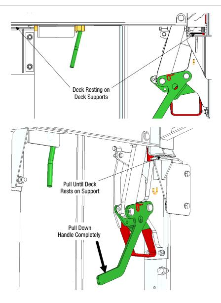
Repeat steps 5-6 for the other side of the deck. The deck is now in the lowered position. The Deck Level Indicator on the outside of the car will show the deck is in the lowered position.
