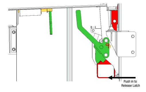
While the Latch is still disengaged, pull the Deck Lift Handle down to the mid-point. It may naturally release to this position.
