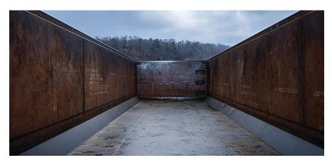
they're harder to unload. With this design, the slab self-centers, reducing damage and failure. This shape also allows for much easier car cleanout for other services such as scrap. There is no need to get into corners, because lading settles into the middle.
